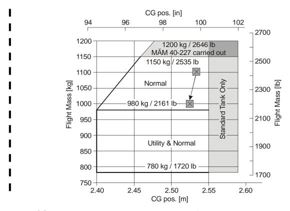
The CG's shown in the diagram are those that from the example in Table 6.4.3 - CALCULATION OF LOADING CONDITION.
