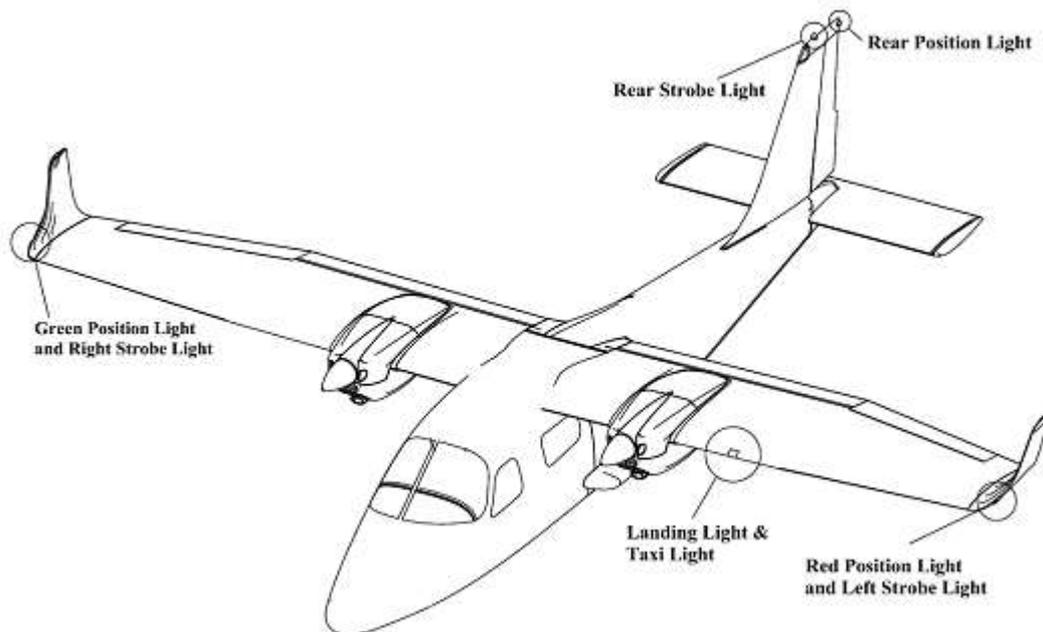
Figure 10. – External lights arrangement
