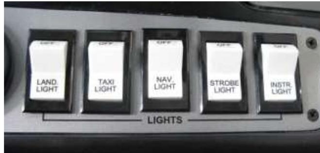
**Figure 11. – Lights switches panel**
