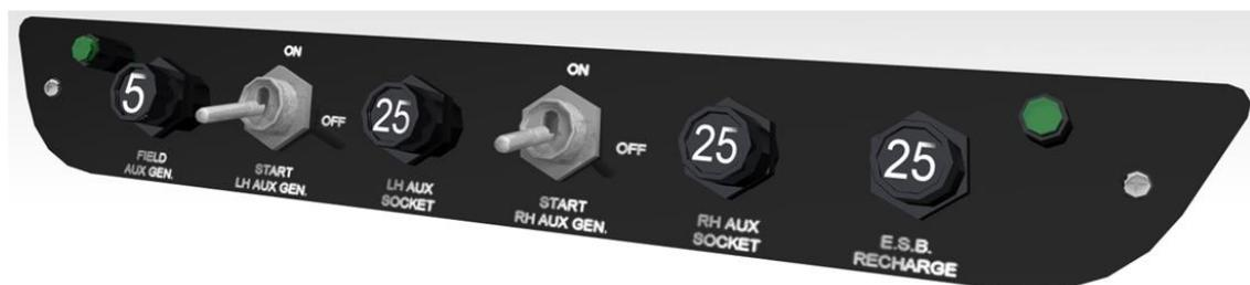
**LH breakers rack: built-in generators field switches and system related breakers (panel type 2)**
