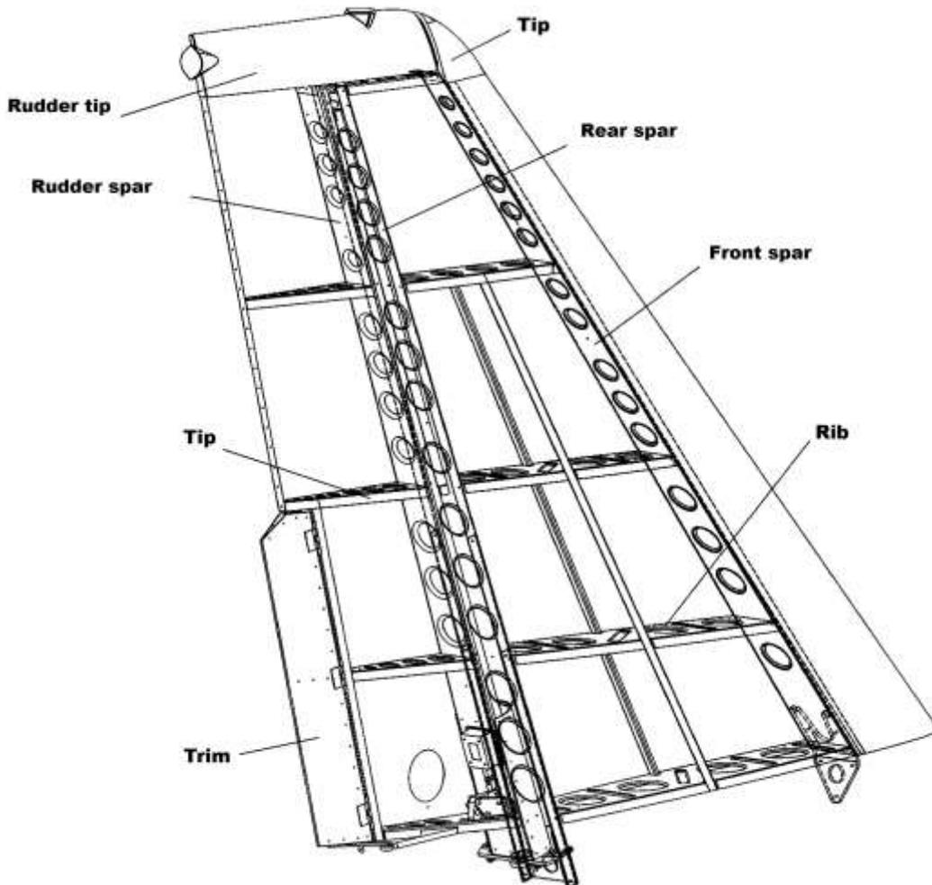
Figure 3. – Vertical empennage structure
