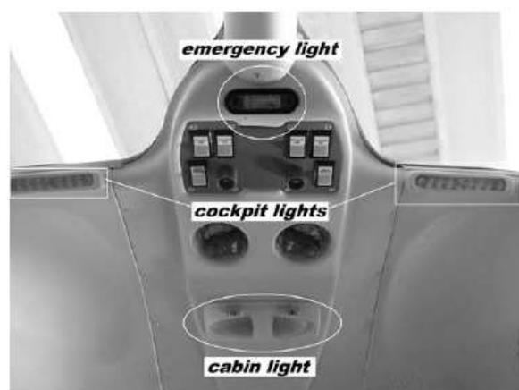
Figure 9. – Over-head panel lights arrangement
