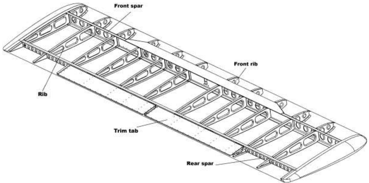
Figure 4. – Stabilator structure
