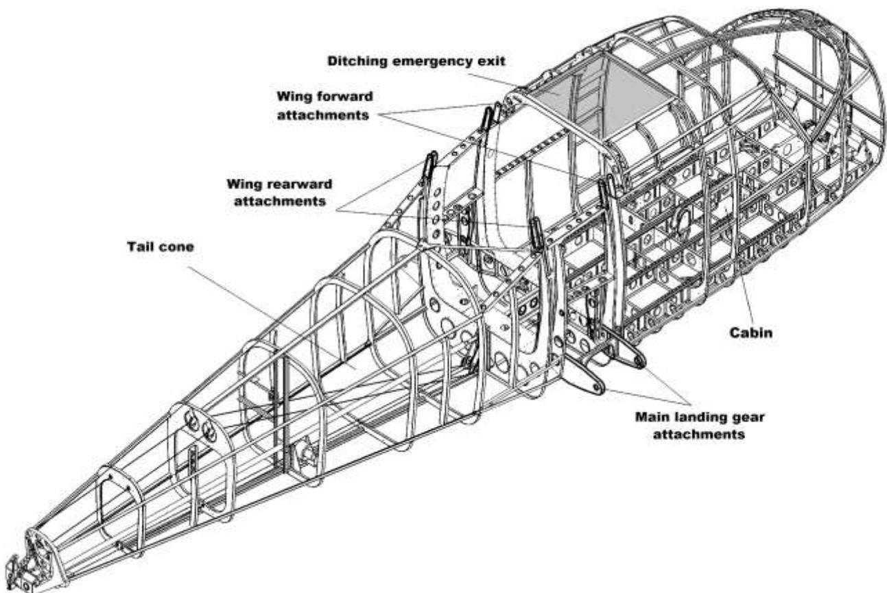
Figure 2. – Fuselage structure
